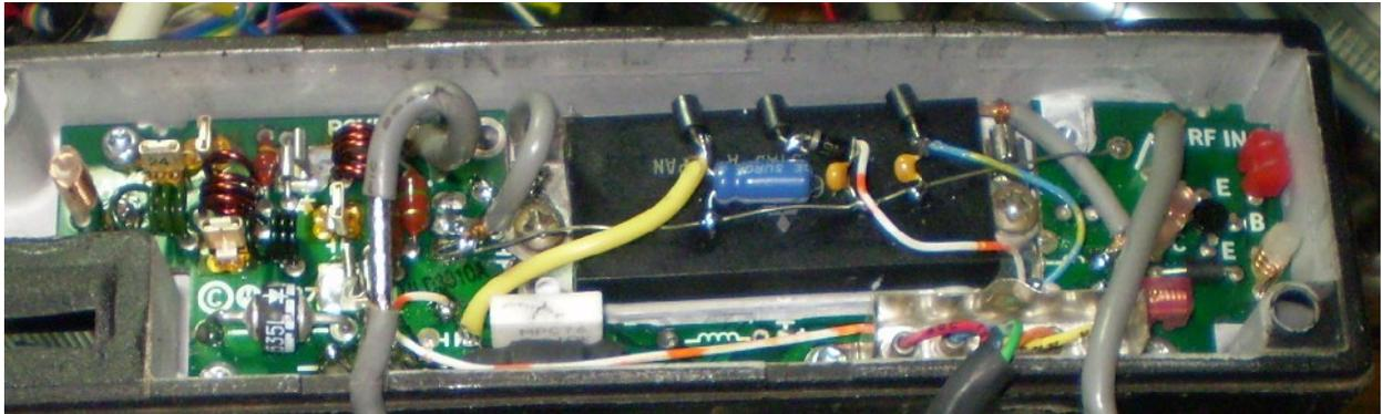
Some additional tweaking of L2462, L2461 and L2460 may be done until maximum power output is achieved as observed on a watt meter.
