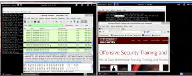
Fig. 5. A malicious virtual machine running macof on an Open vSwitch virtual network and successfully sniffing HTTP traffic with Wireshark from another tenant virtual machine.
