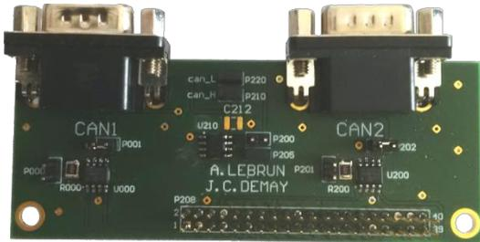
**Figure 9. Picture of the unpopulated PCB of the CANSPY extension board (v1.3)**
