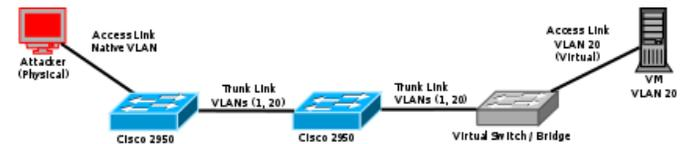
The second scenario as depicted in *Figure 6* still uses a physical Kali 2.0 system for the attack, however only a single physical switch sits in between the attacker and the virtual network.
