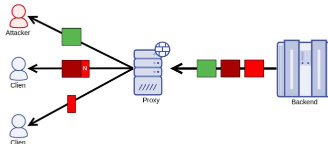
Figure 14. The smuggled response is splitted by the Proxy, as the Content-Length header is smaller than the message body. The extra bytes are controlled by the attacker and build a new malicious response.
